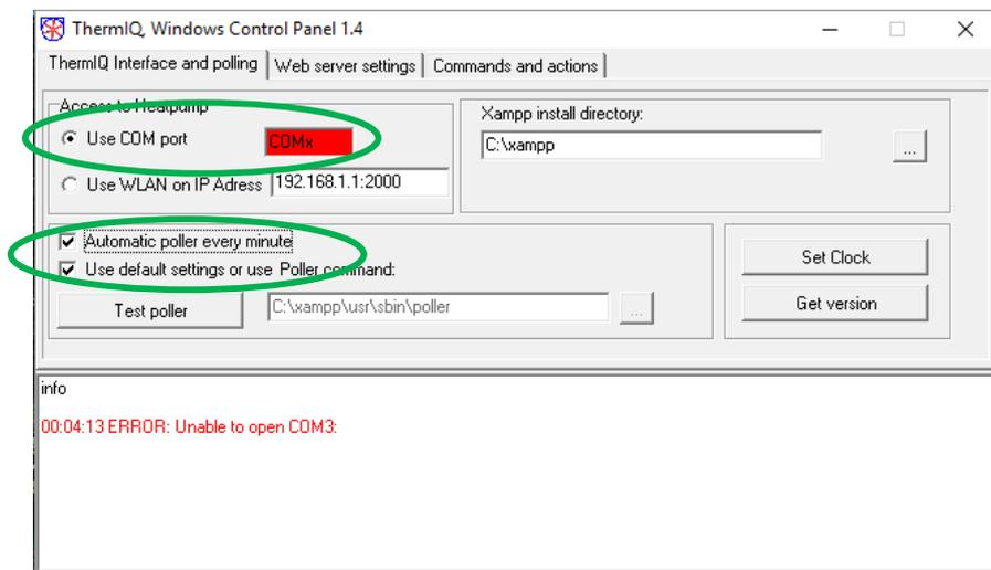
Fill in the right COM-port from above and make sure both tick-boxes are checked. The Control-panel must always be running in order for ThermIQ to collect data.
